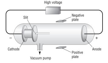
8. Thomson observed that the production of cathode rays did not depend on the kind of gas in the tube or the type of metal used for the electrodes. What
